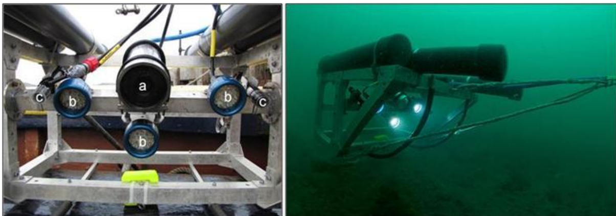
Figure 2.1: Flying array used for the towed video survey. a = high definition video camera, b = LED lights, c = lasers
