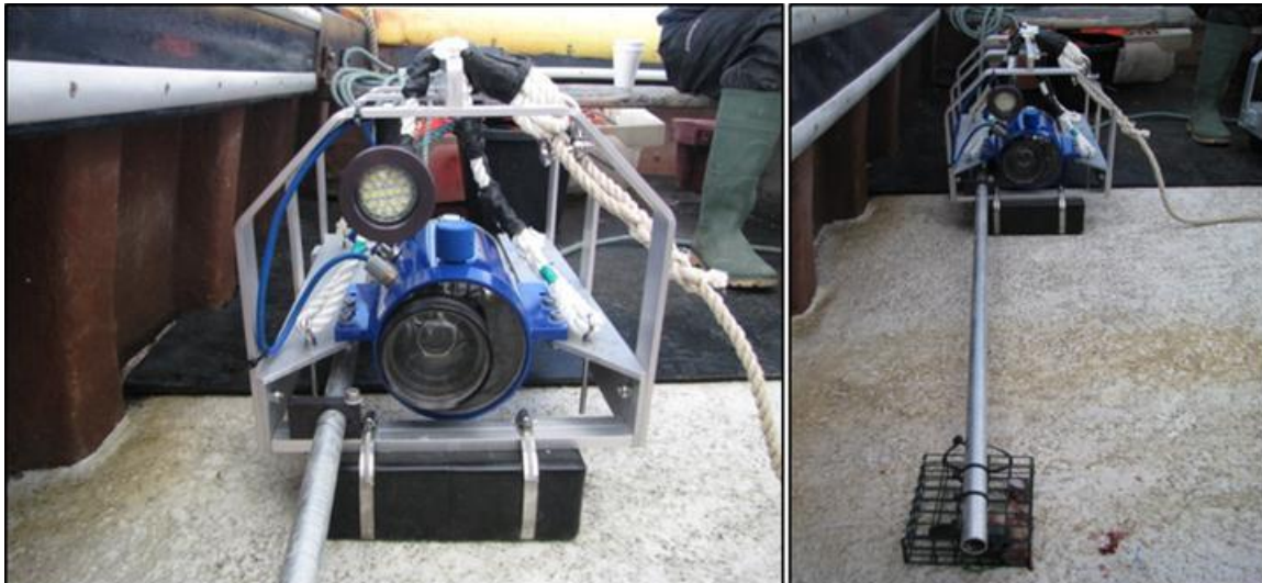
Figure 2.2: BRUV static frame with bait box developed for the 2011 survey
